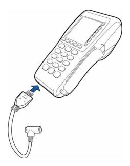
Figure 4 Power Adapter Cable Connection to a V<sup>x</sup>670 Terminal
